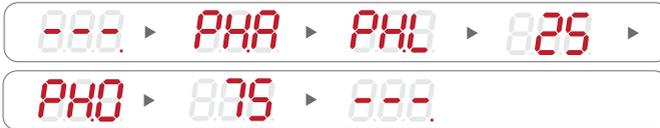
When positive high voltage alarm activated, green LED will turn-on at top-right corner and red LED will blink with audio alarm at the alarm status as below.
