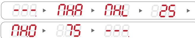
When negative high voltage alarm activated, green LED will turn-on at top-right corner and red LED will blink with audio alarm at the alarm status as below.
